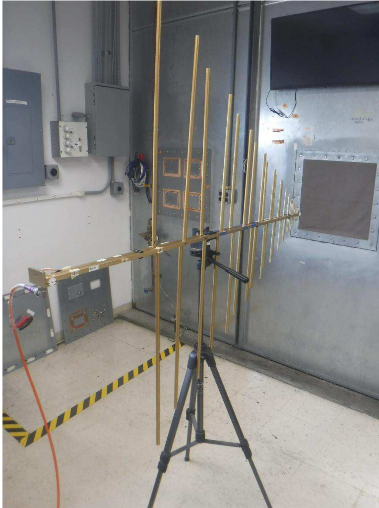
Photograph 12. Test Sample (LPA Vertical Tx)
